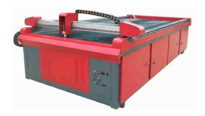
Input voltage – 415V 3Ph 50/60Hz Cutting speed – 0-12000mm/min Transmission way – USB Operation format – G code and HPGI Dimensions – 2200 x 3850mm
